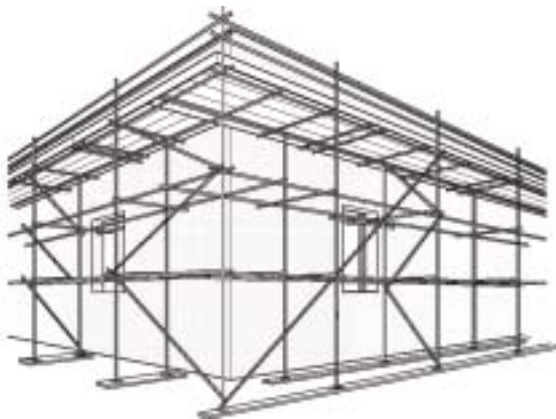
Typical independent tied scaffolding.
