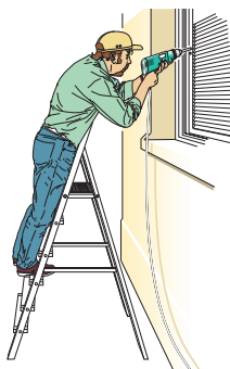
Figure 2b Correct - steps facing work activity
